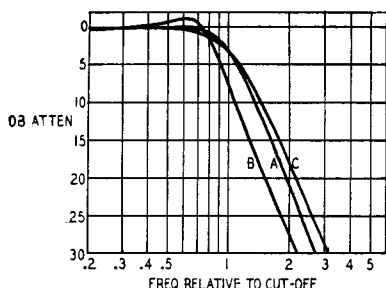
Fig. 908. Response curve of the low-frequency section of the crossover network of Fig. 906-b. Curve A is usually published for the values shown; curve B is the actual curve of the filter feeding load R , with a source impedance of zero; curve C is the response with values for a constant-resistance filter.
